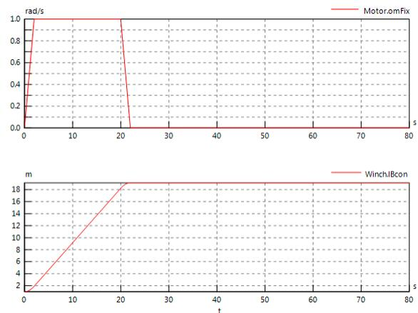
Because of prefilled pressure in hydraulic circuit the tensioner cylinder is initially fully extracted and then tensioned by the winch when the vessel is in motion. The cylinder extraction is shown in the figure below. When the tensioning system is in operation the cylinder is oscillating 1.5 meters which is one fourth of the vessel movement due to the gear ratio given by the topology of the tensioning system.
