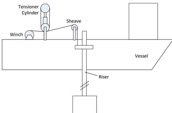
The figure above shows a simplified riser tensioning system on a floating production vessel holding with the purpose to keep constant tension in the riser.
