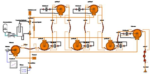
The model contains a combination of elements from the Hydraulic, 1D Mechanics, Planar Mechanics and Belt Drives library together with control signal boxes.
