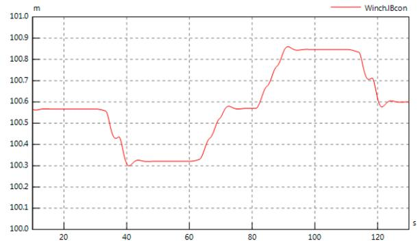
It is here demonstrated how SimulationX® can be applied for simulating winch systems. The model can easily be changed and expanded to i.e. a electrical drive instead. And more complex control algorithms can be tested through simulation.
