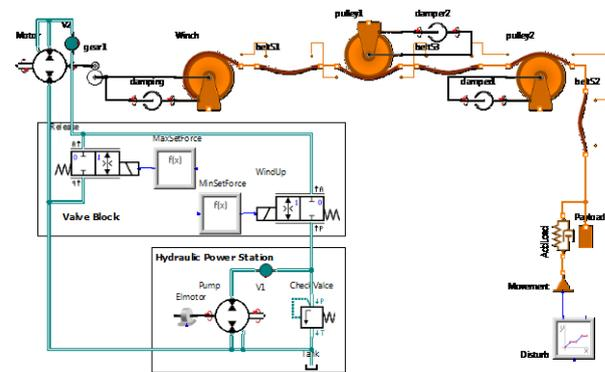
The model contains a combination of elements from the Hydraulic, 1D Rotational Mechanics, 2D Planar Mechanics, 3D MBS Mechanics and Belt Drives libraries together with control signal boxes. The winch is connected through a gearbox to a hydraulic motor. The two valves are controlled by a sensor measuring the torque on the winch and they either bypass the motor or supply oil to wind-in the winch.
