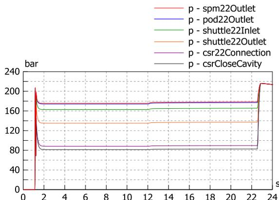
This shows the pressure transients for «Close» line for the CSR between the pod's SPM valve to the valve actuator's "Close cavity" before optimization begins. We see very clearly that the high pressure losses are across the shuttle valve and the pipe length from the shuttle valve to the actuator gate. The same plot is made for the actuator's "Open" line.
