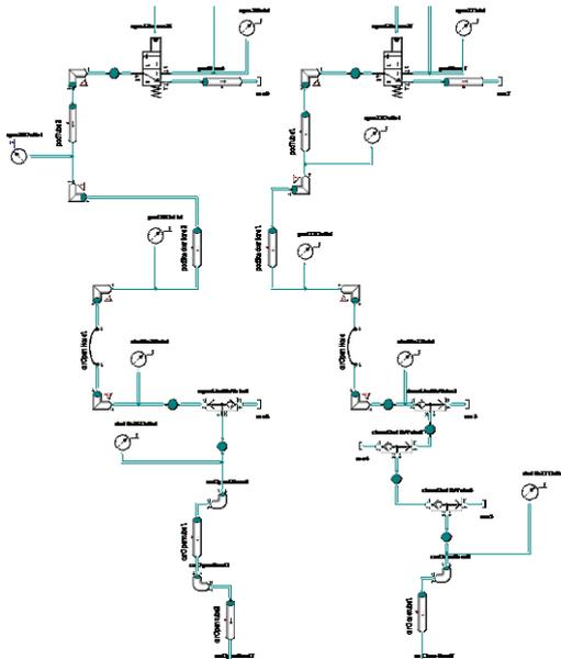
The model of the control lines are made using elements from the standard library, and have a high level of detail. In addition, pressure gauges are placed in the system model, so that pressure transients in the lines can be plotted and items with high losses can be identified.
