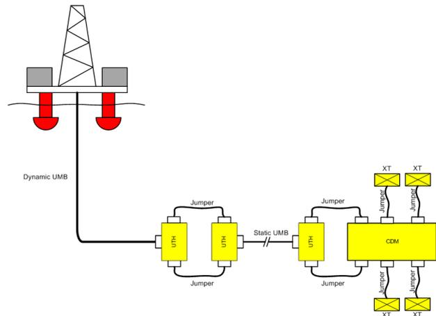
Figur 1 Subsea control system for oil and gas production
