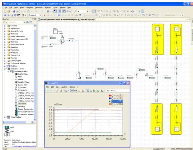
Figure 2 SimulationX<sup>®</sup> model of an injection system
