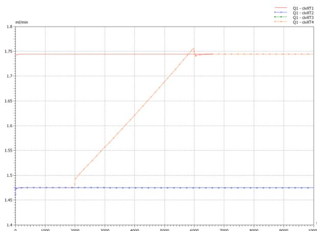
Figure 5 Change in the injection rate with a variable throttle valve
